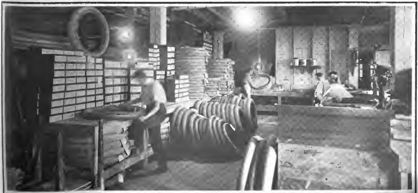
Shawmut Tires, Both Shoes and Inner Tubes, Undergo a Rigid Inspection Before Leaving the Factory
